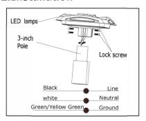
1) Connect the AC wire of the lamp as shown in the picture, then insert the lamp into the 3-lnch pole.
