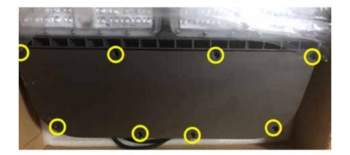
3. Loosen the screws which holds the driver (circled in yellow below)
