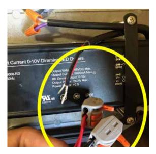
Cut the power wires from the driver, leaving enough lead to connect the replacement driver, and for Altech Electronics to duly perform a Root Cause Analysis of the returned driver (circled in yellow below)
